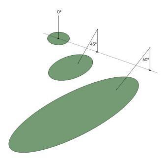
A simple FOV calculator for determining target dimensions based on infrared radiometer model, mounting height, and mounting angle, is available on the Apogee website: <a href="https://www.apogeeinstruments.com/irr-calculators">https://www.apogeeinstruments.com/irr-calculators</a>.
