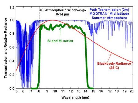
Spectral response of SIL series infrared radiometers. Spectral response (green line) is determined by the germanium filter and corresponds closely to the atmospheric window of 8-14  $\mu$ m, minimizing interference from atmospheric absorption/emission bands (blue line) below 8  $\mu$ m and above 14  $\mu$ m. Typical terrestrial surfaces have temperatures that yield maximum radiation emission within the atmospheric window, as shown by the blackbody curve for a radiator at 28 C (red line).
