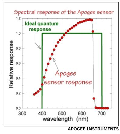
short of laboratory accuracy. They are relatively insensitive to light below 440 nm and overly sensitive to light in the 550 to 650 nm range. They do not measure red light over 650 nm.
