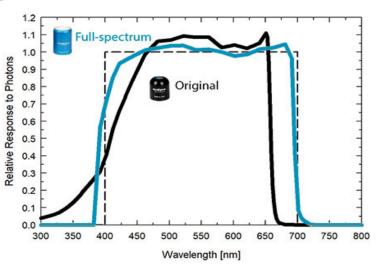
Mean **spectral response** measurements of six replicate Apogee MQ-210 and MQ-510 series quantum sensors.
