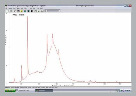
The detector collects light for the spectroradiometer via fiber-optic cable. The spectroradiometer then transmits its measurements to a PC where custom software (included) displays the spectrum of the light source. Live data can be saved as a data file suitable for work in other programs, such as Excel or SigmaPlot.
