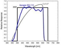
GaAsP photodiodes cutoff at approximately 650 nm and are more sensitive to longer (red) versus shorter (blue) wavelengths
