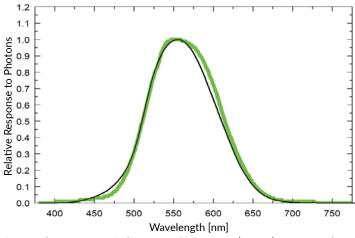
Spectral response of photometric sensors (green) compared to the CIE 1931 photopic curve.
