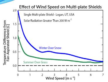
Naturally-aspirated shields are subject to significant measurement errors when wind speeds are less than  $3 \, \mathrm{m \ s^{-1}}$ . Errors increase when snow covers ground surface.
