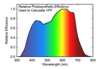
In addition to the ability to measure YPFD, spectroradiometers more accurately measure PPFD than quantum sensors because they measure radiation intensity at multiple wavelengths and are calibrated at each of these wavelengths, eliminating spectral errors caused by sensor spectral sensitivity. Fortunately, recent advances allow spectral measurements to be made underwater at a much lower cost than a few years ago (http://www.apogeeinstruments.com/field-spectroradiometers/).
